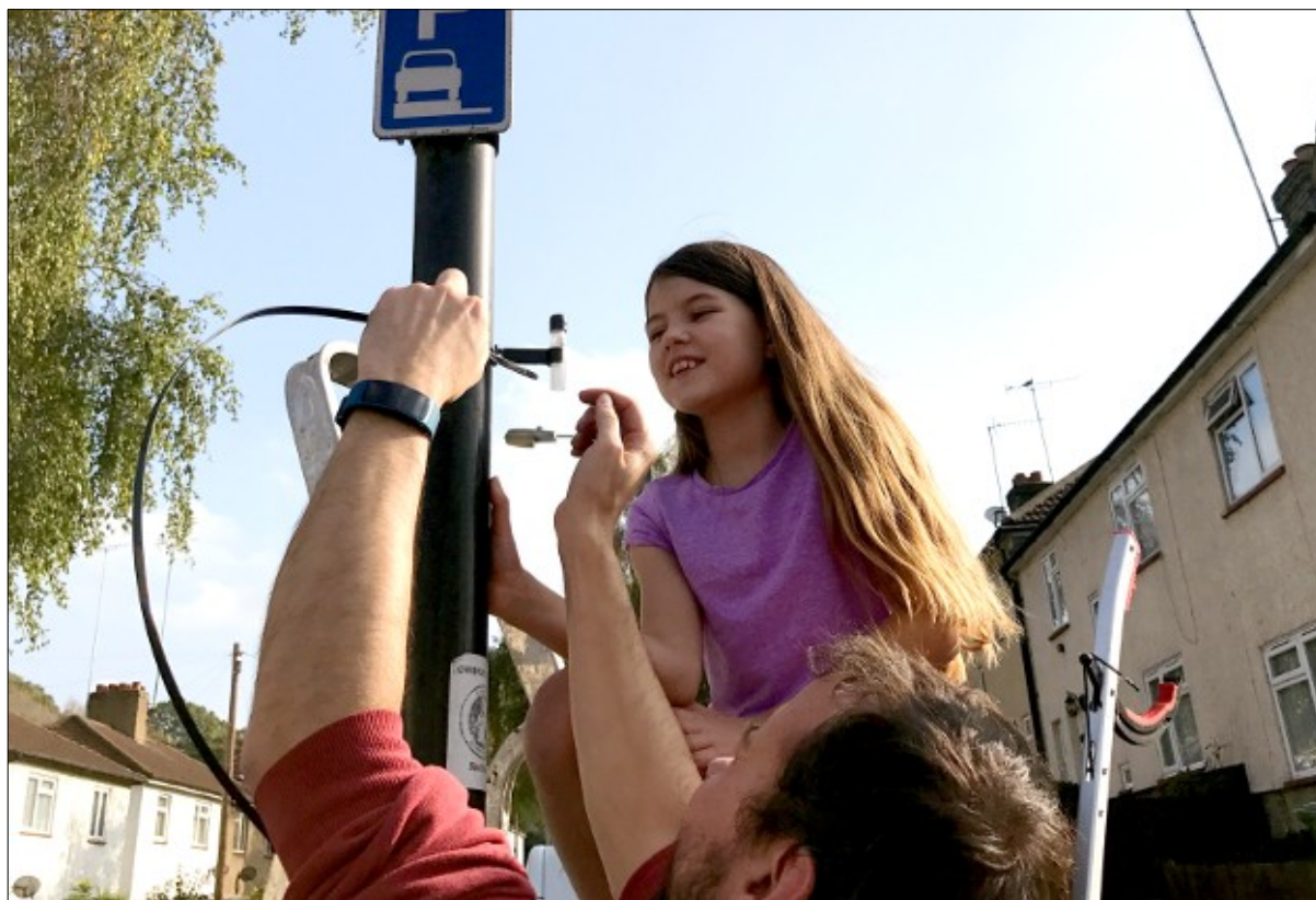
Photo: Residents of Charlton in the London borough of Greenwich install diffusion tubes for measuring air pollution. A cable tie is used to secure a clip which holds the diffusion tube.
